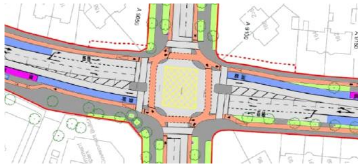
Figure 5-3 - - Example of Junction Type 3 from BCPDG
