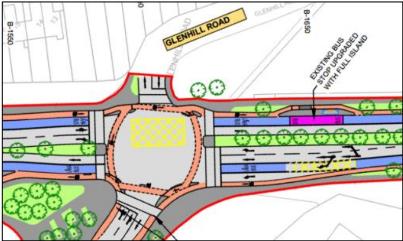
Figure 5-2: Junction Type 2 Proposed Glenhill Road Junction
