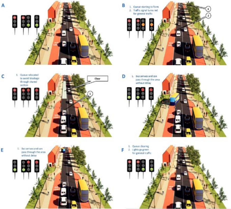
Figure 12-5: Signal Controlled Bus Priority Schematic Operation
